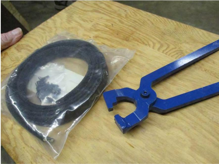
**Have you ever had trouble setting split rivets when applying radiator shell lacing? With this tool it is a snap!**
