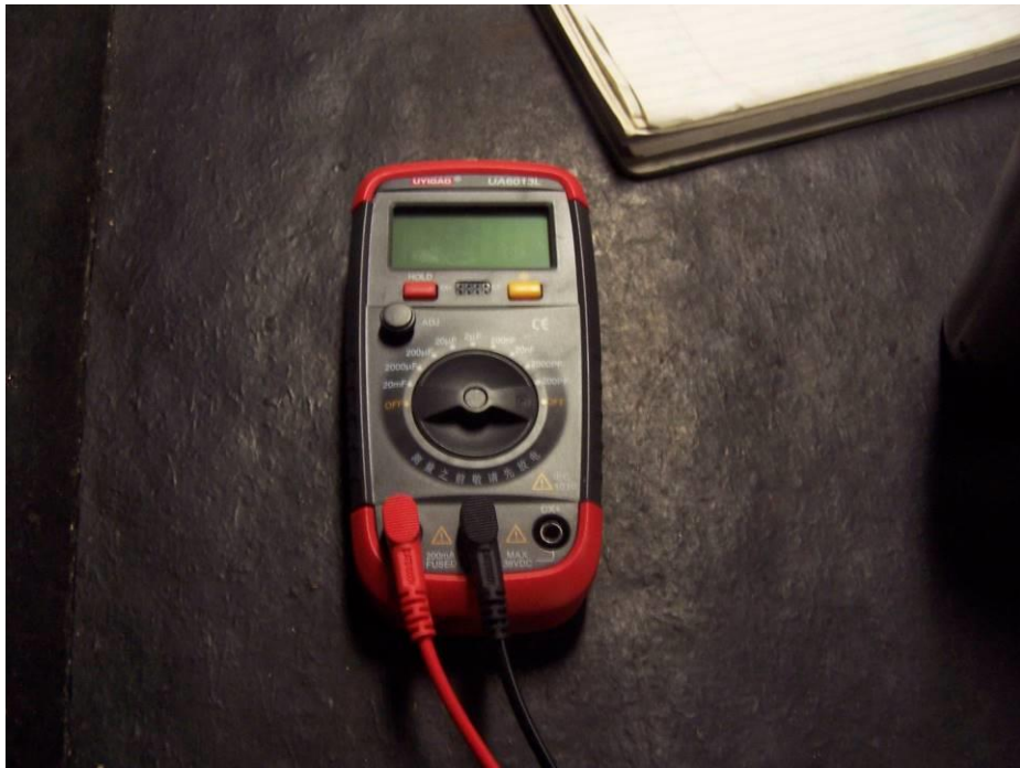
This is what the capacitor meter to check condensers looks Like.
