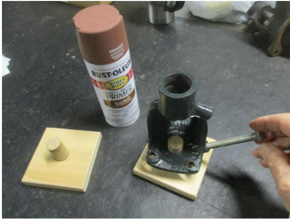
A jig to hold the castings during painting, made by Bobby.
